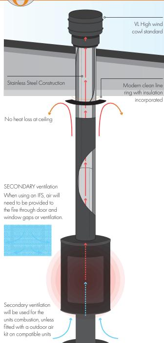
The VisionLINE Insulated Flue System (IFS) replaces traditional air-cooled flue designs with high-quality CE Approved Ceramic insulation, ensuring the outer skin remains cool while safely passing through combustible areas. By eliminating the need for ventilated skins, IFS prevents heat loss and retains valuable room air, enhancing energy efficiency.
