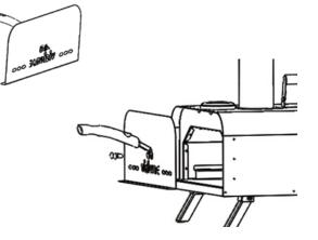
4. Attach handle to pellet burn basket with 2 x bolt and 2 x nut. Nut goes to inside of basket.
