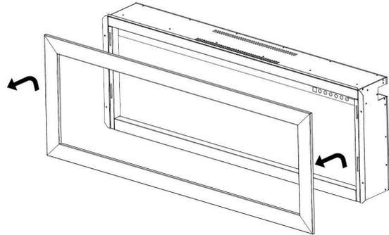
2. Locate and carefully remove glass retainer screws one at a time.
