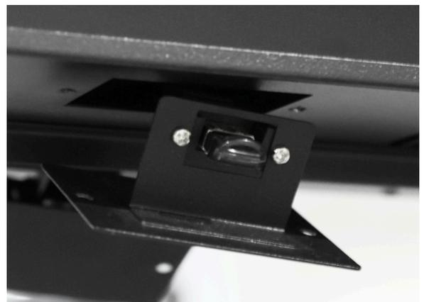
5. Remove the thumb drive and upload the chosen video file from the Visionline website onto it. You can then plug it back into your Vesta fireplace and re-assemble it.
