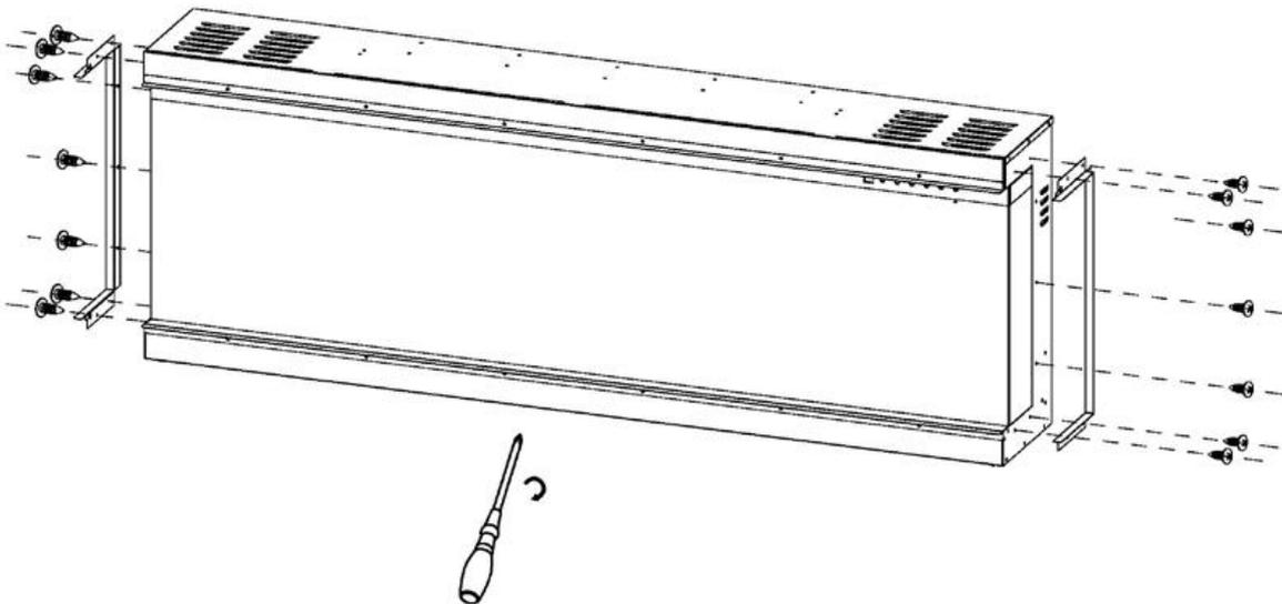
4. Remove the screws from the fireplace as shown in the picture below.
