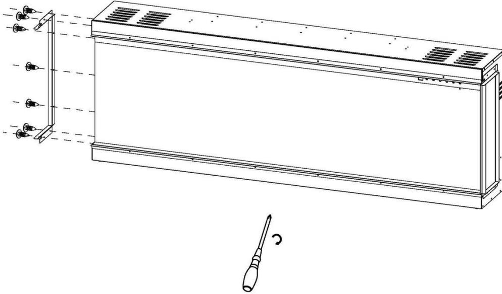
4. Remove the screws from the fireplace as shown in the picture below.
