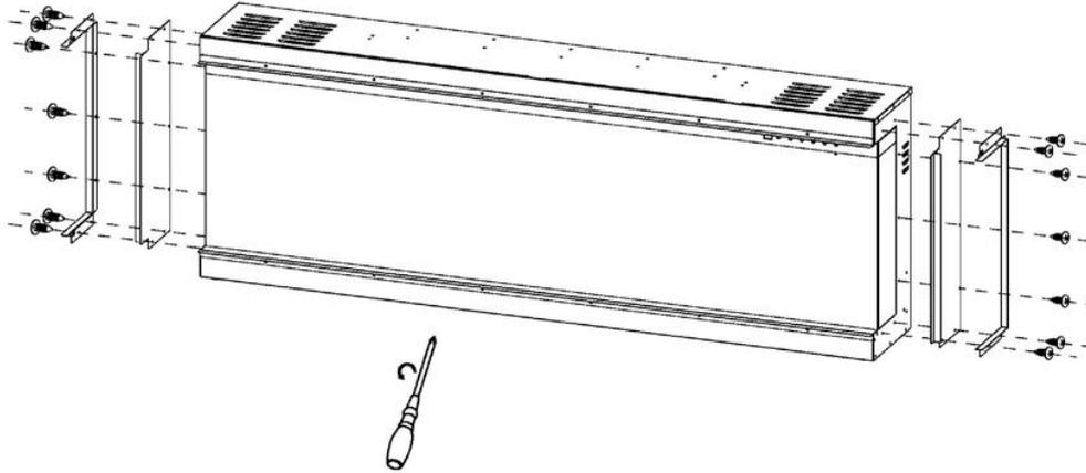
3. Fix back the fending bars after the panels are removed.
