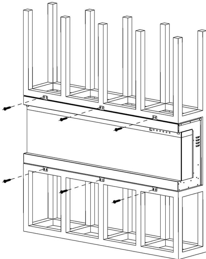
8. Cover the glass panel with protective plastic bag and install plywood or drywall.
