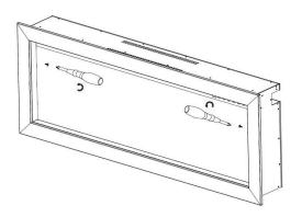
2. Locate and carefully remove glass retainer screws one at a time.
